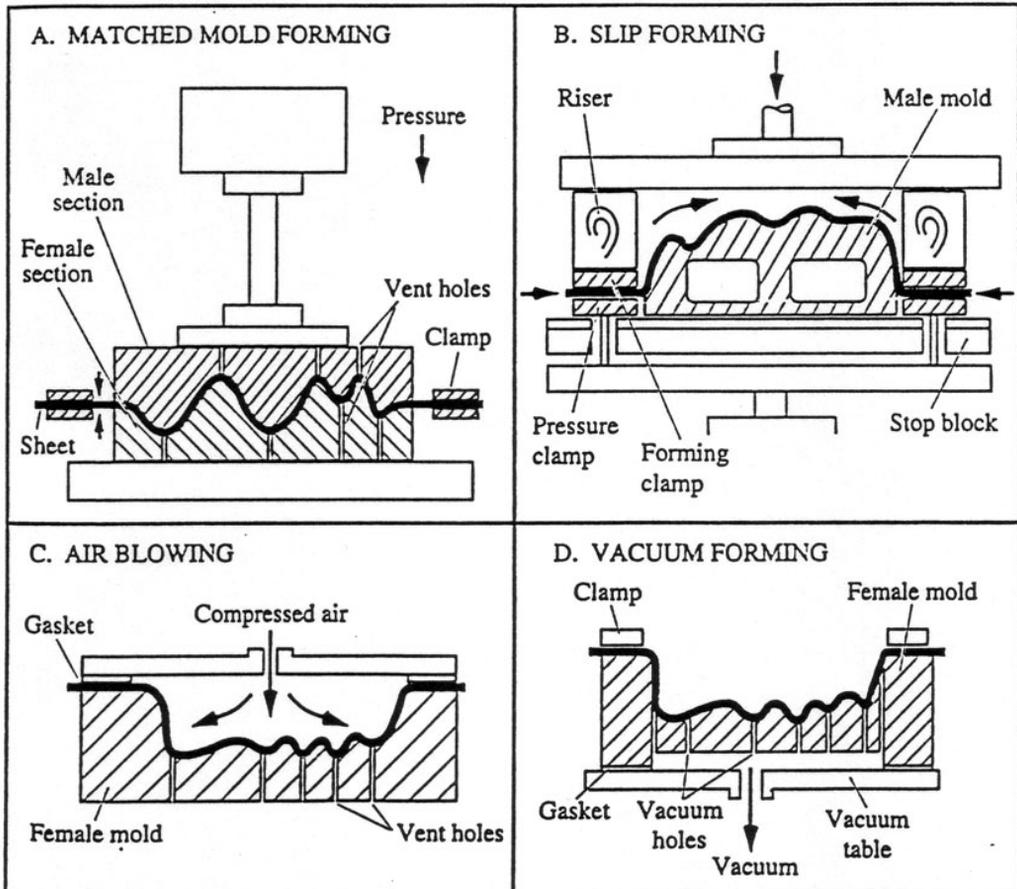
Fig. 10-2 Thermoforming classifications [2].
