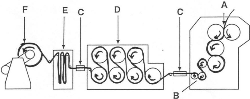
**Figure 1.5** Schematic view of an inverted "L" calender plant for the production of plastic sheeting. Molten polymer is dropped into the calender system at A. Continuous sheet is formed by passing the melt between the rolls. One of the surfaces is given texture by an embossing roll, B. Thickness gauges, C, provide data for control of the process. The sheet is cooled, D, tensioned using wind-up accumulators, E, and accu-accumulated on the wind-up roll, F (Holmes-Walker, 1975).
