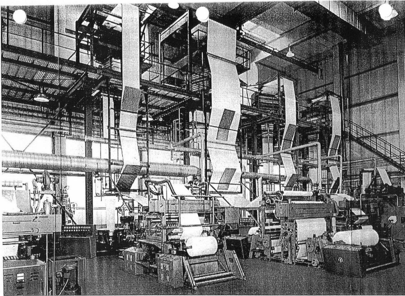
Figure 37. High-output line for LDPE blown film. (Photo: Windmüller und Hölscher, Lengerich, West Germany)
