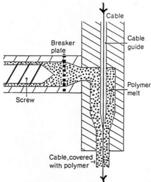
Combination of Poiseuille flow (pressure driven) and Couette (drag) flow due to the moving wire.
