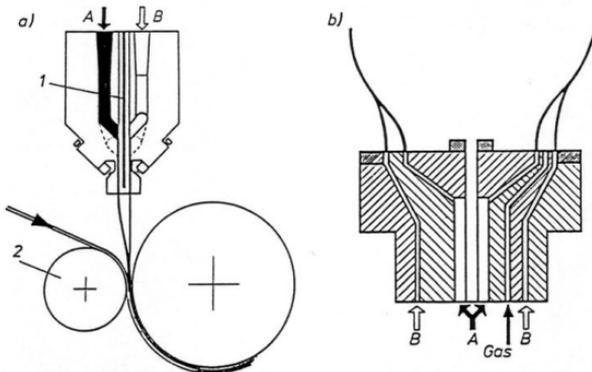
Dual slot coextrusion dies, a) Flat slit die, 1 Heat separation, 2 Pressure roll, b) Blown film die
