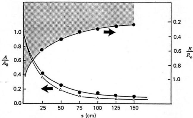
**Fig. 15.1** Melt strand area and radius profiles in the melt drawdown region: ●, nylon 6 at 265°C and takeup velocity of 300 m/min; △, PP at 262°C and takeup velocity of 350 m/min. (Reprinted with permission from H. F. Mark, in *Rheology*, Vol. 4, F. R. Eirich, ed., Academic Press, New York, 1969.)
