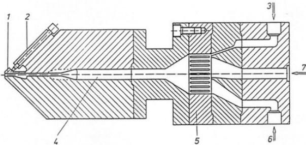
Fig. 6.2 Feed block (System Dow) for bringing melt streams together before the flat slit die. 1 Flex lip, 2 Pressure bolt, 3 Cover layer material, 4 Melt channel with a flow restrictor, 5 Adapter, 6 Base layer material, 7 Main layer material
