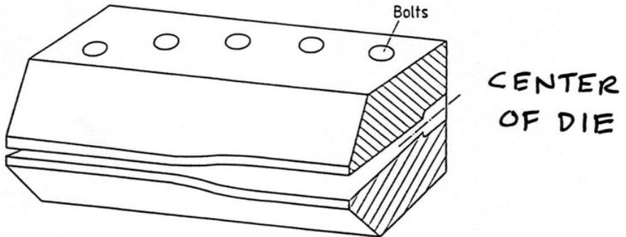
Clam shelling due to internal pressure in a flat slit die
