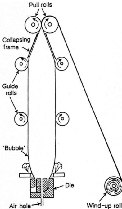
Fig. 7.2. Die, 'bubble', and take-off equipment in a film blowing unit.
