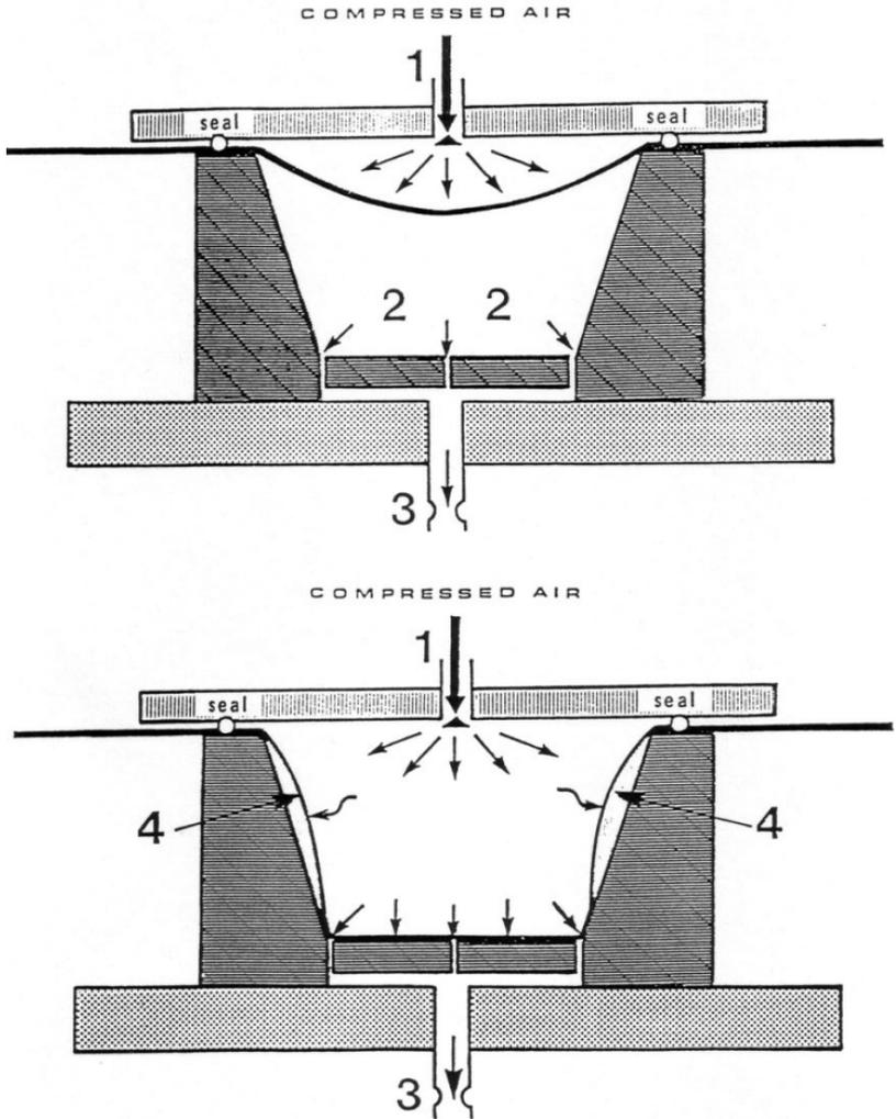
FIGURE 76 Overpressurized forming condition: (1) incoming pressure force; (2) undersized or small number of vent/vacuum holes; (3) restricted vent/vacuum channel; (4) trapped air pockets.
