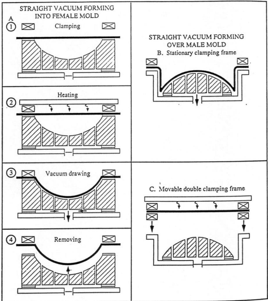
Fig. 10-8 Methods of straight vacuum forming [2].
