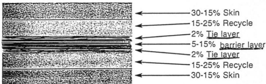
Figure 5-3 Typical coextruded structures containing recycled material in additional layers. (a) Six-layer asymmetrical structure. (b) Seven-layer symmetrical structure. Courtesy: Dow Chemical Company.
