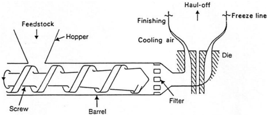
Fig. 7.1. Extruder and die in a film blowing unit (after Cogswell).
