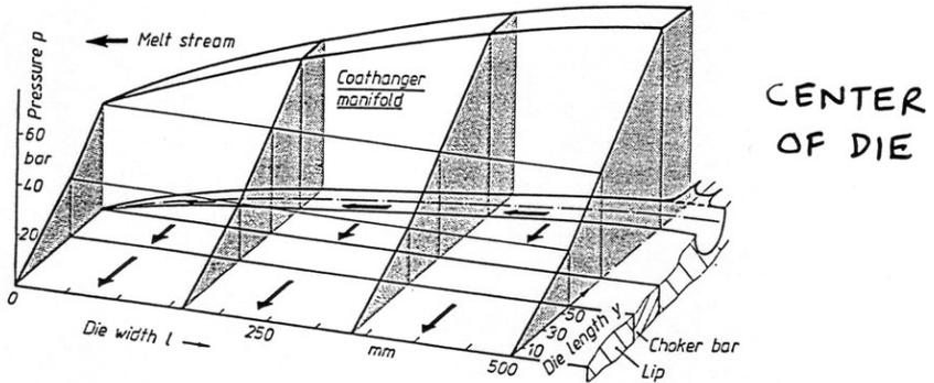
Typical pressure distribution in a flat slit die
