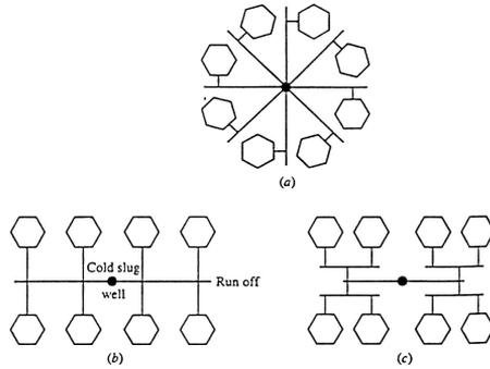
Figure 1: Two naturally balanced (symmetric) runner systems and one counter-example.
