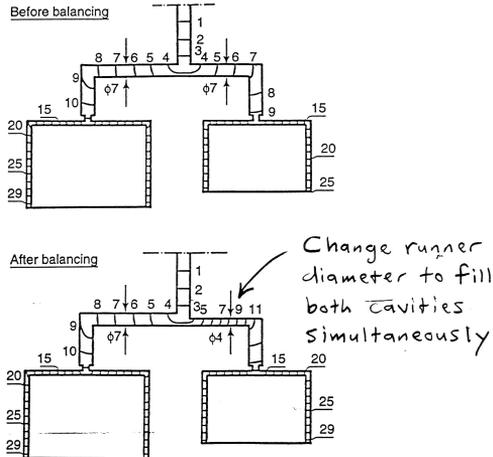
Figure 2: An artificially balanced runner system.
