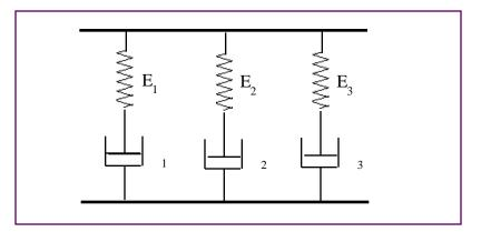
$E(t) = \underbrace{0}_{0}^{1} \exp(-\frac{t}{0}) + \underbrace{0}_{0}^{2} \exp(-\frac{t}{0}) + \underbrace{0}_{0}^{3} \exp(-\frac{t}{0})$ Or, in general  $E(t) = E_{n} \exp(-\frac{t}{t_{n}}) \text{ where } E_{n} = \underbrace{0}_{n}^{0}$
