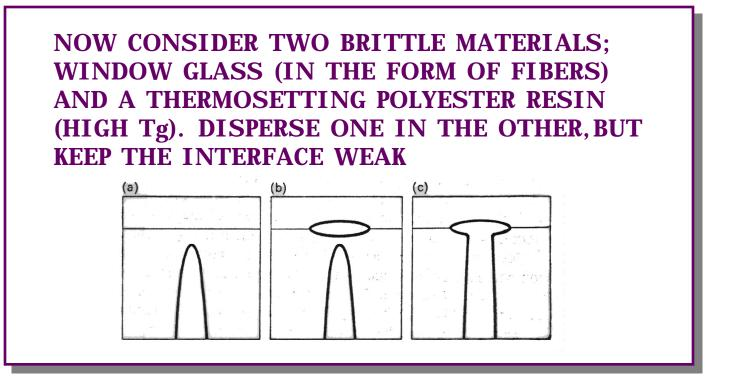
NOTE: CRACK STOPPING IS NOT THE ONLY "TOUGHENING" OR ENERGY ABSORPTION MECHANISM. YOU SHOULD KNOW WHAT CRAZING AND YIELDING ARE
