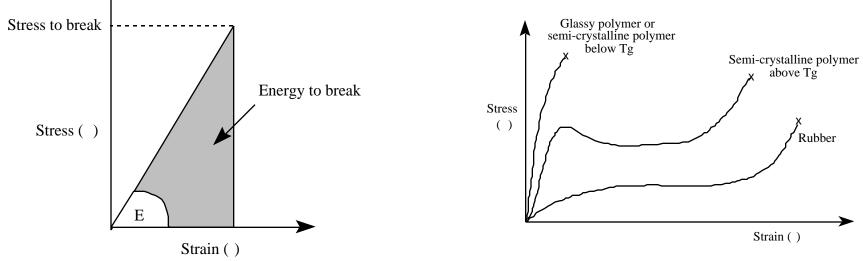
Many of the mechanical characteristics of polymers that we have just discussed (Eg strength, stiffness, toughness, yield behaviour) can be determined from Stress/strain measurements.
