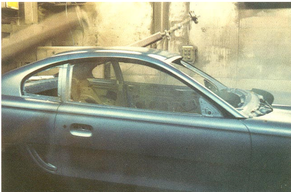
Conductive nanocomposites can assist electrostatic painting of automotive parts. (Photo: Visteon.)
