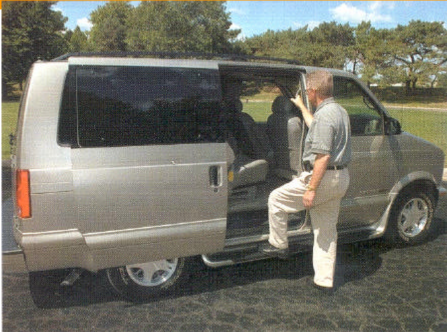
General Motors' 2002 Safaro and Astrp vans represent the commercial debut of polyolefin nanocomposites, appearing in the TPO step assist.
