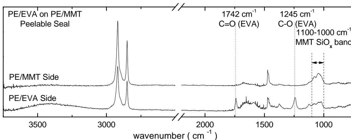
**Figure S4.** ATR-FTIR of fracture seal surfaces (25.4 mm wide flat seals, 1000 psi/8 s). Spectra from peelable seals between PE/EVA and PE/MMT, where MMT nanofillers are detected on the PE/EVA side whereas no EVA is detected on the PE/MMT side. This result qualitatively indicates that the PE/MMT interfacial adhesion, mediated by LLDPE-*graft*-MAH, is weaker than the adhesion between PE and EVA, mediated by polymer entanglements and, to a smaller extent, by co-crystallization.
