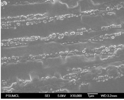
Fig 1. SEM micrographs of aligned BaTiO<sub>3</sub> (10 V%) particles in cured PDMS. A 1.6 kV/mm a.c field at 100 Hz is used for alignment. The frequency is chosen to minimize the space charge at the electrodes that screens the applied field and to limit electrophoretic transport of the filler phase.
