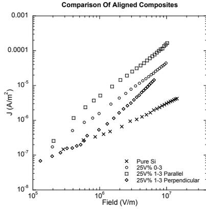
Fig 3: Current-Voltage characteristics of aligned composites. It is evident that the conduction is highest in the case of z-aligned composites while x-y aligned shows a slightly lower conduction compared to 0-3 composites.
