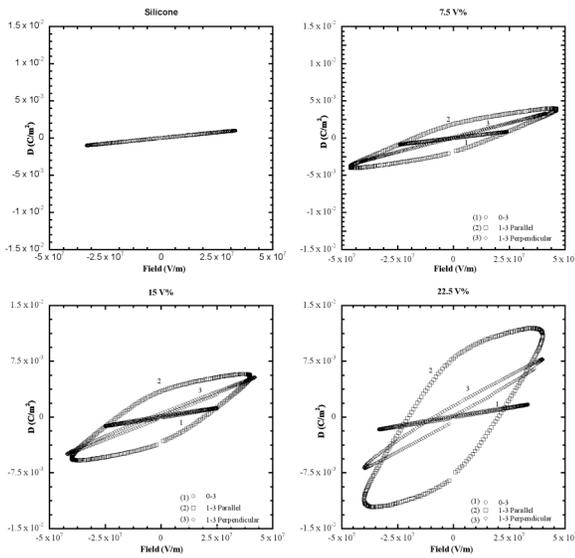
Fig 4: A comparison between the polarization-electric field loops, obtained at 10 Hz, for various volume fractions of structured and randomly dispersed composites. The z-aligned composites clearly indicate higher losses compared to 0-3 and x-y aligned.
