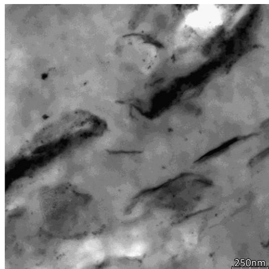
**Fig. 10.** A TEM image of MgAlO at 10% loading in EVA highlighting the composite morphology at the tactoids length scale.
