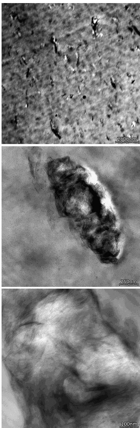
**Fig. 9.** Hierarchical composite morphology of EVA with 5% MgAlO. TEM images at: low magnification (top, highlighting the micrometer scale dispersion of filler assemblies), medium magnification (middle, showing the LDH tactoid structure as swollen by EVA), and higher magnification (bottom, showing the dispersion of individual LDH layers at the nanoscale).
