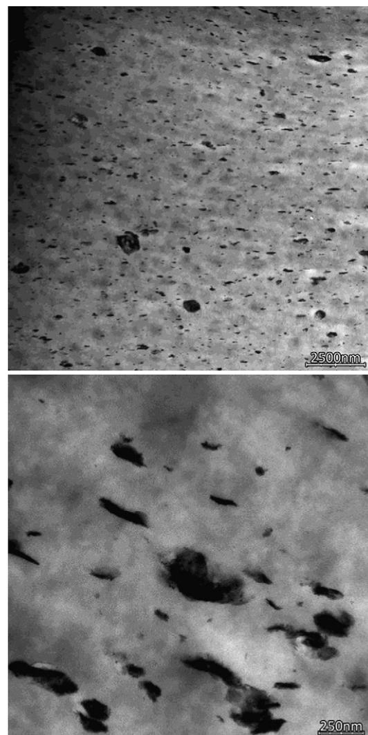
**Fig. 11.** Low magnification images of ZnAlO in EVA at 10% loading highlighting the dispersion at the micrometer scale and the tactoids' size. Compared to the MgAlO these composites show tactoids which are much smaller (better dispersion at the micrometer scale) but much more compact (less swollen by EVA, indicating worse nanometer scale dispersion).
