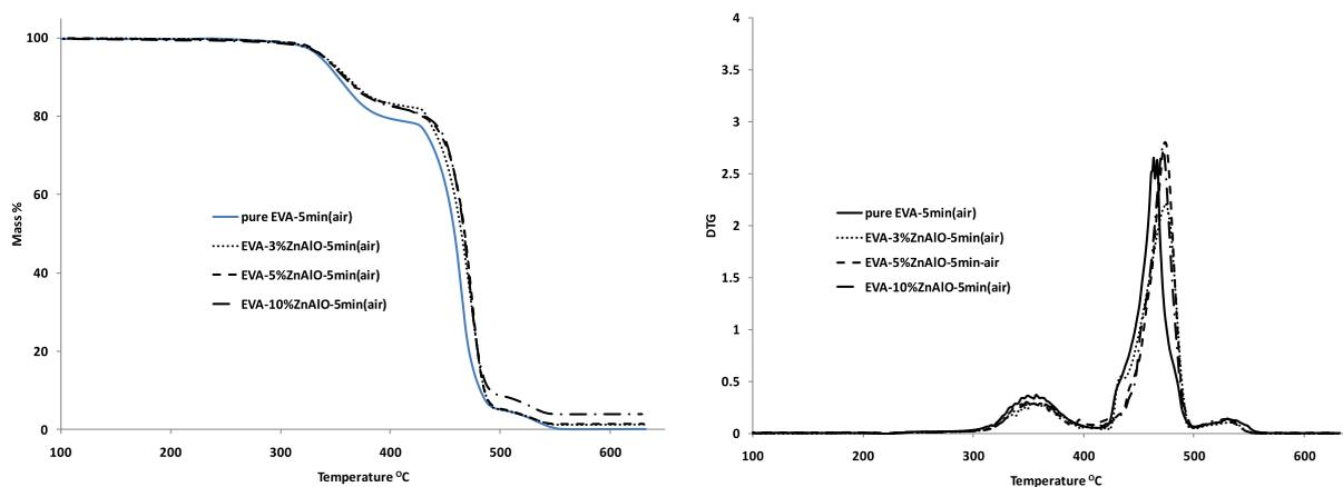
Fig. 12. TGA and DTG curves for EVA and its composites with ZnAlO-LDH.
