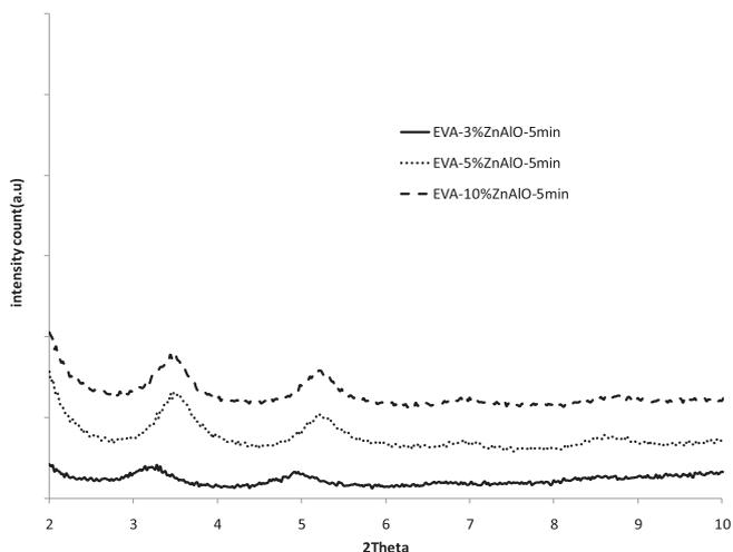
Fig. 5. XRD traces of EVA/ZnAlO-LDH composites at 5 min time for melt blending.
