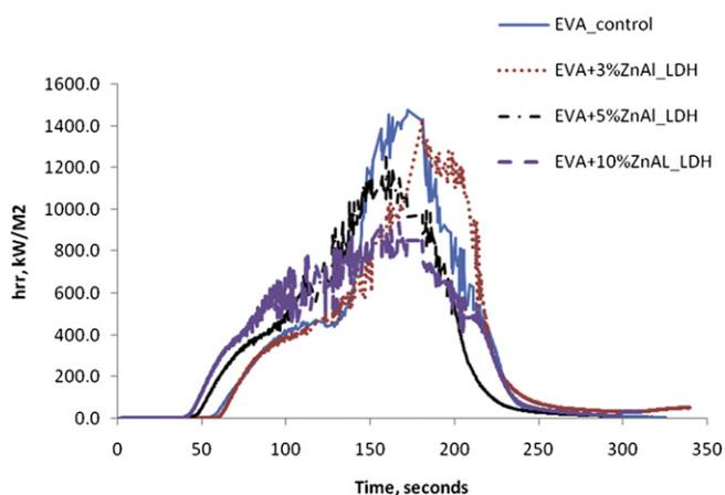
Fig. 19. Heat release rate curves for EVA and its composites with ZnAlO.
