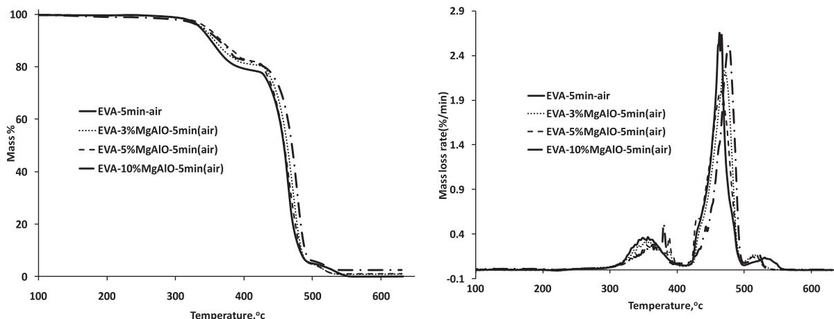
Fig. 13. TGA and DTG curves for EVA and its composites with MgAlO-LDH.
