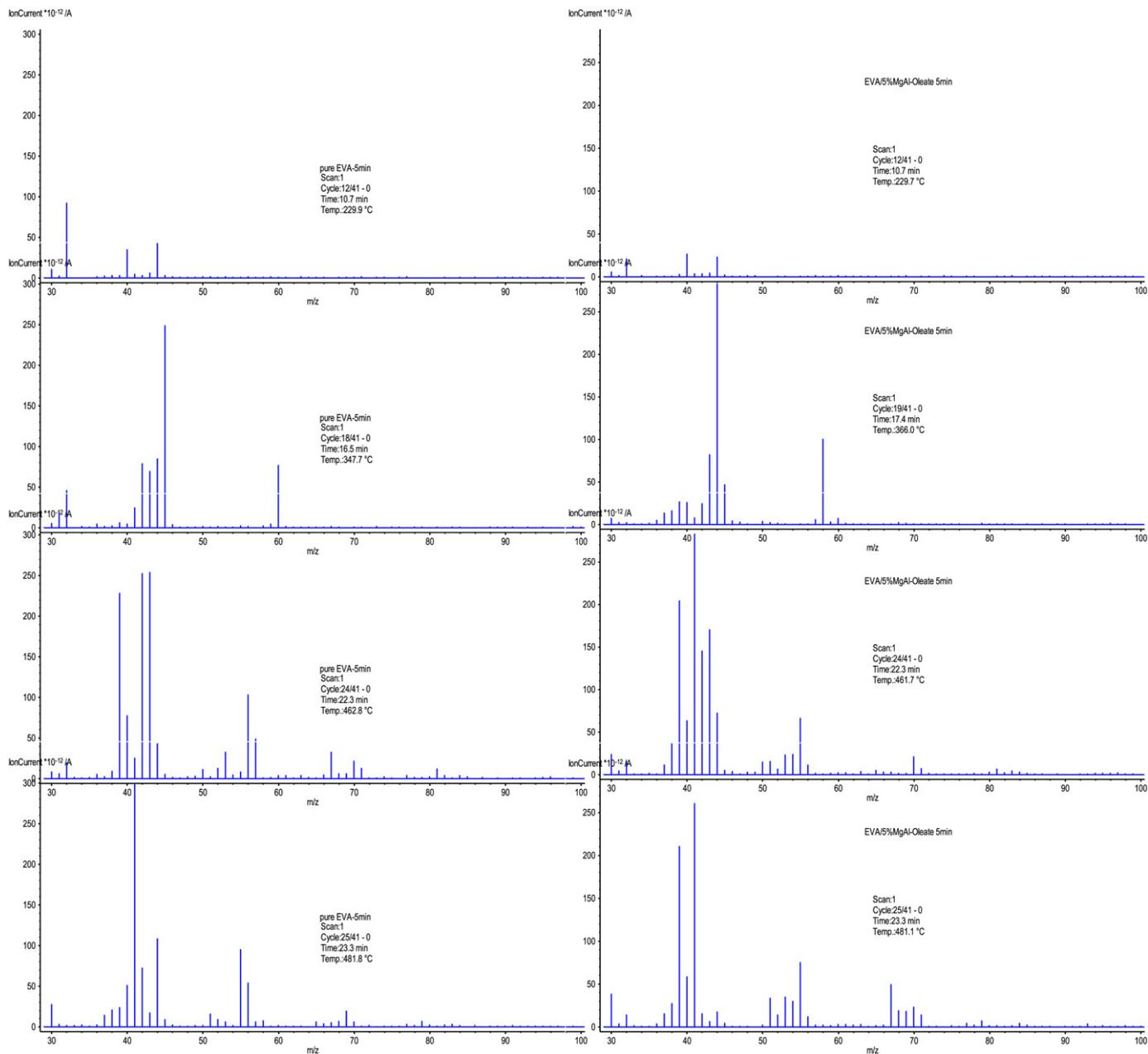
Fig. 16. Mass spectra for several temperature ranges in the degradation of both pristine EVA and its composites with 5% MgAlO.
