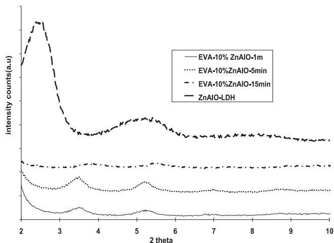
Fig. 7. Effect on XRD trace for ZnAlO-EVA at various times of melt blending. The top trace is that of the LDH, and the time of melt blending increases from 1 min to 5 min–15 min for the lower curves.
