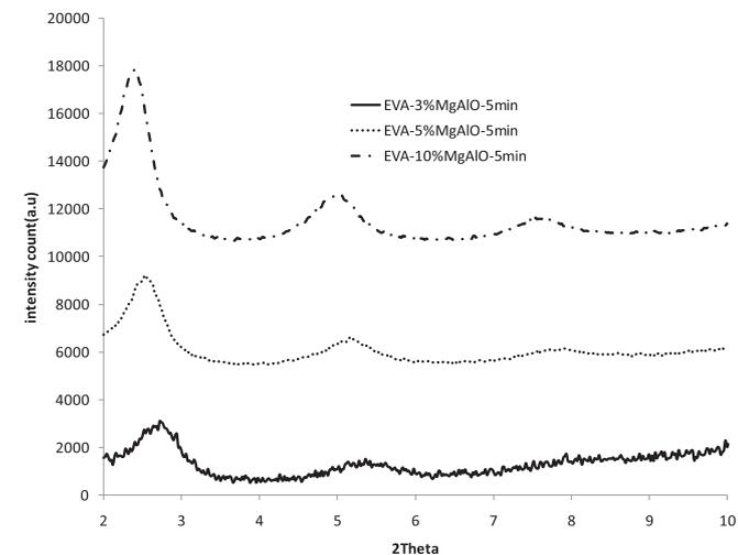
Fig. 6. XRD traces of EVA/MgAlO-LDH composites at 5 min time for melt blending.
