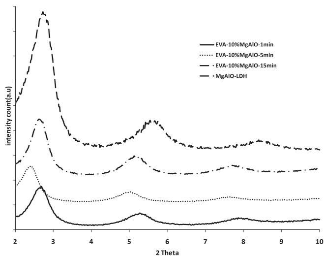
Fig. 8. Effect on the XRD trace for MgAlO-EVA at various times of melt blending. The top trace is that of the LDH, and the time of melt blending increases from 1 min to 5 min–15 min for the lower curves.
