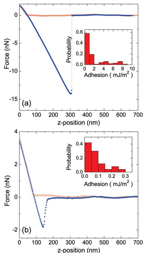
**Figure 3.** (a) Representative force–distance approach (red circles) and retraction (blue circles) curves for the bitumen film from Utah oil sands collected in a 1 mM KCl aqueous solution. Inset shows the adhesion histogram. (b) Representative force–distance approach (red circles) and retraction (blue circles) curves for the bitumen film from Utah oil sands collected in the ionic liquid (IL). Inset shows the adhesion histogram.
