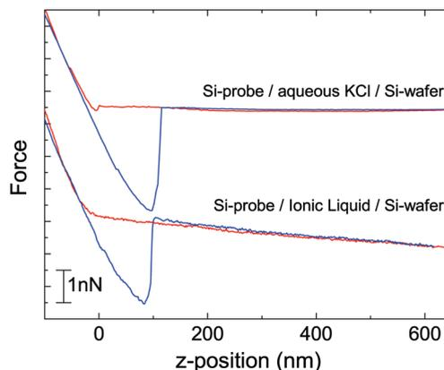
**Figure 6.** Force–distance atomic force microscopy (AFM) curves of a colloidal silica probe and a silicon-surface immersed in 1 mM KCl aqueous solution and in [bmim][BF<sub>4</sub>] IL (the lines are shifted for the sake of clarity, and the long-range approach forces are contrasted, in water versus in IL). There are no measurable long-range forces in aqueous KCl, whereas there is a systematic attraction in IL, acting over hundreds of nanometers above the silicon-wafer surface.
