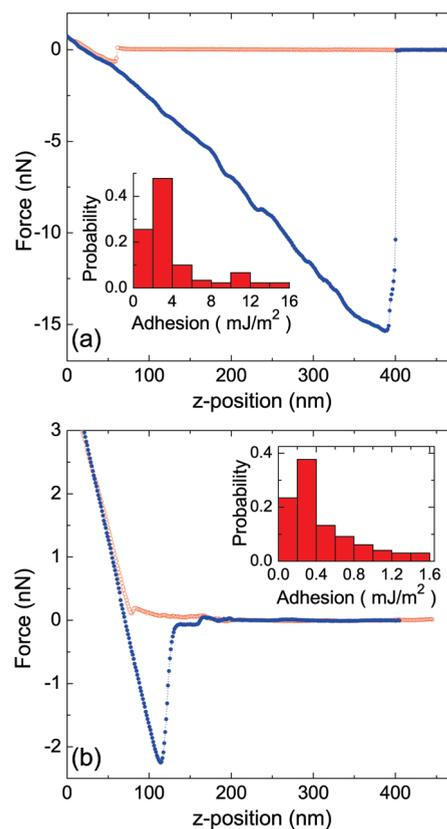
**Figure 4.** (A) Representative force–distance approach (red circles) and retraction (blue circles) curves for the bitumen film from Alberta tar sands collected in the 1 mM KCl aqueous solution. Inset shows the adhesion histogram. (B) Representative force–distance approach (red circles) and retraction (blue circles) curves for the bitumen film from Alberta tar sands collected in the IL. Inset shows the adhesion histogram.
