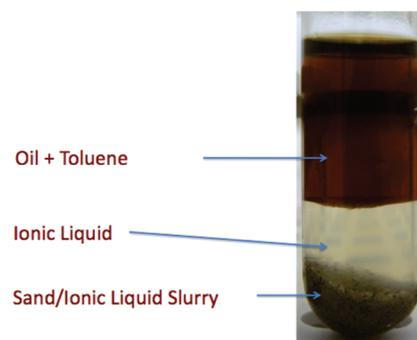
**Figure 1.** Photograph showing the phases formed by mixing an oil/sand mixture with 1-butyl-2,3-dimethyl-imidazolium borontetrafluoride ([bmmim][BF<sub>4</sub>]) and toluene in the proportions 1:2:3 at room temperature.
