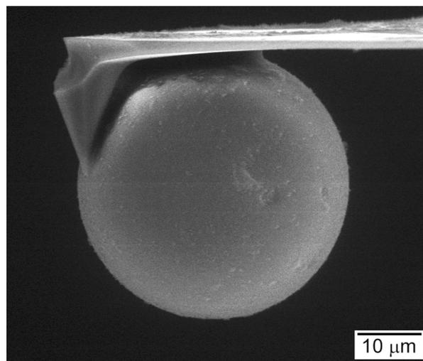
**Figure 2.** Scanning electron microscopy (SEM) photomicrograph of the silica colloidal probe attached on the AFM tip (diameter of sphere = 43.6  $\mu$ m, viz, a contact area of 1  $\mu$ m<sup>2</sup>), facilitating the measurement of surface forces, rather than the AFM-typical atomic forces measured by sharp AFM tips.
