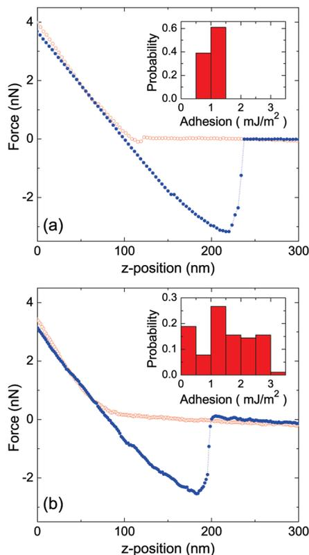
**Figure 5.** (A) Representative force–distance approach (red circles) and retraction (blue circles) curves for the bare silicon wafer collected in the 1 mM KCl aqueous solution. Inset shows the adhesion histogram. (B) Representative force–distance approach (red circles) and retraction (blue circles) curves for the bare silicon wafer collected in the IL. Inset shows the adhesion histogram.
