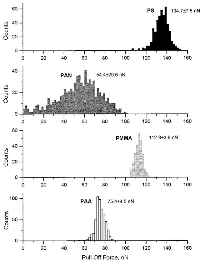
**Figure 6.** Histograms of pull-off forces measured between a polystyrene sphere (radius 3.75  $\mu\text{m}$ ) probe and PS, PAN, PMMA, and PAA surfaces in perfluorodecalin.
