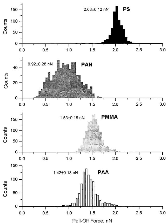
**Figure 5.** Histograms of pull-off forces measured between a gold probe and PS, PAN, PMMA, and PAA surfaces in perfluorodecalin.
