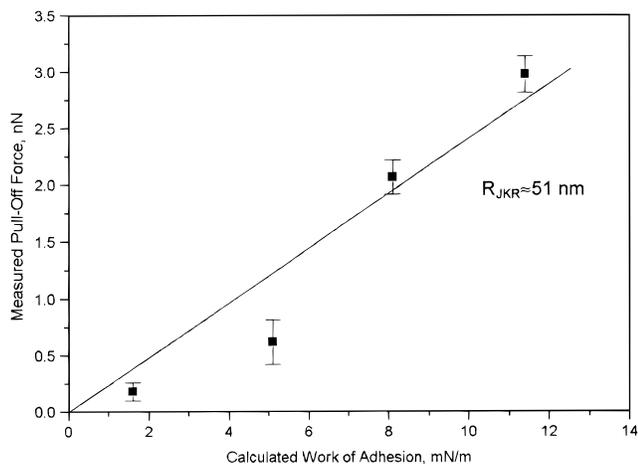
**Figure 3.** Comparison of measured pull-off forces and the calculated work of adhesion for interactions between a  $\text{SiO}_x$  probe and PS, i-PP, PVDF, and FEP surfaces in perfluorodecalin.
