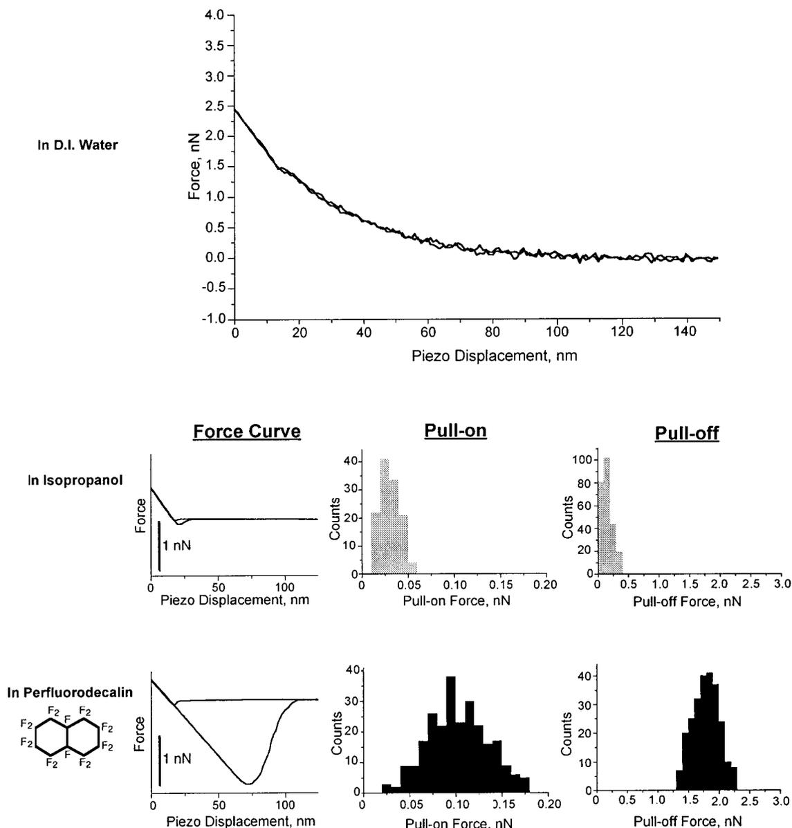
**Figure 1.** Comparison of force curves and pull-on and pull-off forces between a  $\text{SiO}_x$  probe and a PMMA surface in water, 2-propanol, and perfluorodecalin.
