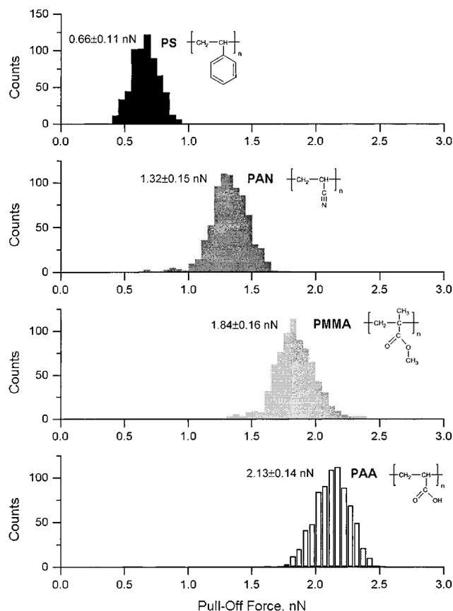
**Figure 4.** Histograms of pull-off forces measured between a  $\text{SiO}_x$  probe and PS, PAN, PMMA, and PAA surfaces in perfluorodecalin.
