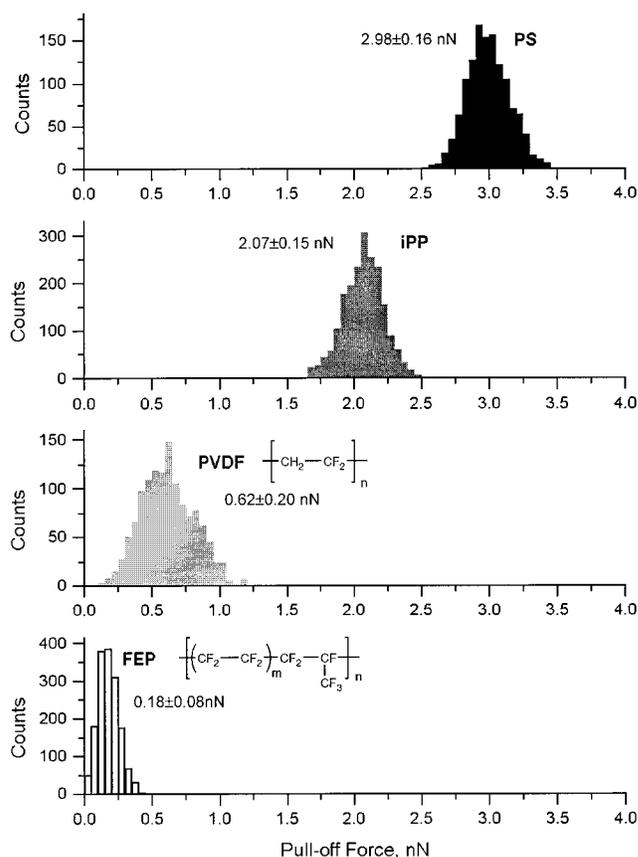
**Figure 2.** Histograms of pull-off forces measured between a SiO<sub>x</sub> probe and PS, i-PP, PVDF, and FEP surfaces in perfluorodecalin.
