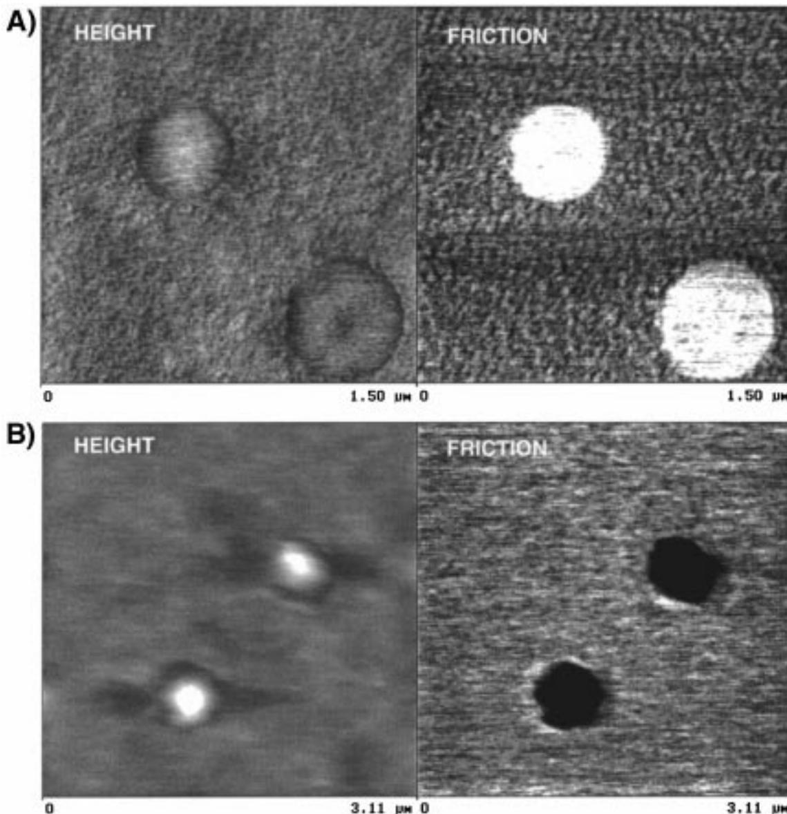
**Figure 7.** Height (AFM) and friction (LFM) images of a spin-cast polystyrene/poly(methyl methacrylate) polymer blend [PS/PMMA (1:10 w/w)], obtained with (a) gold-coated and (b) SiO<sub>x</sub> tips under perfluorodecalin.
