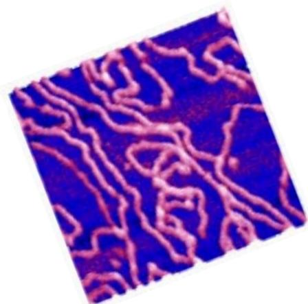
TappingMode avoids the force instabilities caused by thermal drift in contact mode, resulting in time savings and improved image and measurement quality. Stable imaging forces of less than 200pN have been measured during TappingMode operation. Refer to the sidebar (right) for additional discussion of tip-sample forces.
