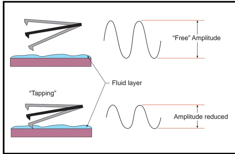
Figure 4: TappingMode cantilever oscillation amplitude in free air and during scanning.
