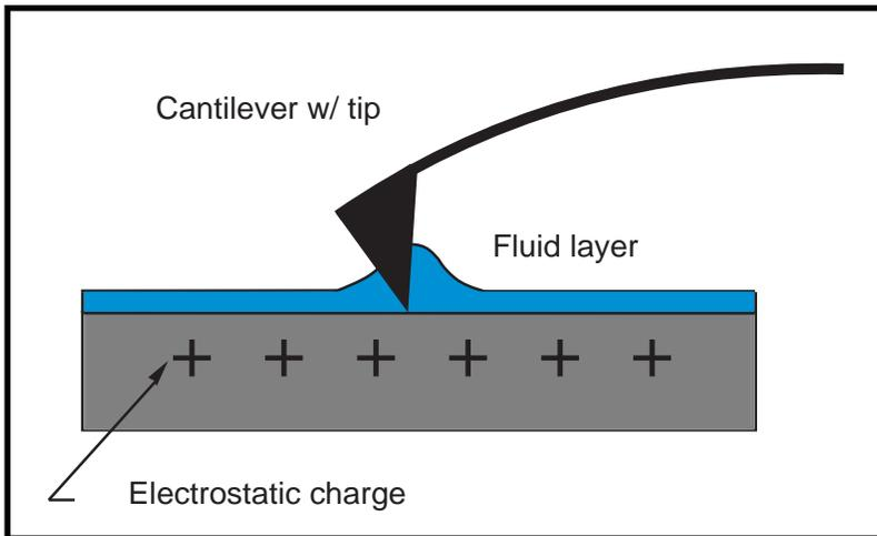
Figure 3: In contact AFM, electrostatic and/or surface tension forces from the adsorbed gas layer pull the scanning tip toward the surface.
