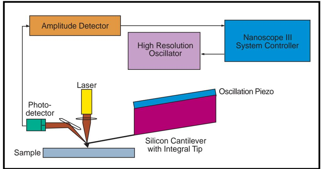
During TappingMode operation, the cantilever oscillation amplitude is maintained constant by a feedback loop (Figure 5). Selection of the optimal oscillation frequency is software-assisted and the force on the sample is automatically set and maintained at the lowest possible level (Table 1 and Figure 6). When the tip passes over a bump in the surface, the cantilever has less room to oscillate and the amplitude of oscillation decreases. Conversely, when the tip
