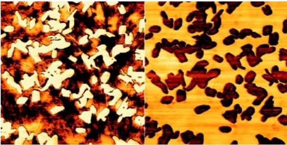
Figure 8: Phase (left) and lateral force (right) images of  $\text{MoO}_3$  crystallites on a  $\text{MoS}_2$  substrate; 6 $\mu\text{m}$  scans. The crystallites show light contrast in the phase image, and dark contrast, corresponding to high friction, in the LFM image. Phase gives superior feature detail, and also shows dark regions on the background likely caused by contamination or adsorbed water. Sample provided by Dr. C.M. Lieber, Harvard University.
