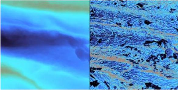
Figure 2: Phase (right) and TappingMode (left) images of wood pulp fiber. The phase image highlights cellulose microfibrils. In addition, a lignin component appears as light areas in the phase image, but is not apparent in the topography image. 3 $\mu$ m scan by Don Chernoff, Advanced Surface Microscopy; sample provided by Dr. Damaris E. Doro Pereira, Aracruz Celulose.
