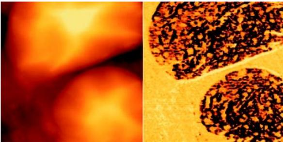
Figure 3: TappingMode (left) and phase (right) images of a composite polymer embedded in a uniform matrix. The high resolution of the phase contrast image highlights the two-component structure of the composite regions. Sample courtesy of Raj Michael.
