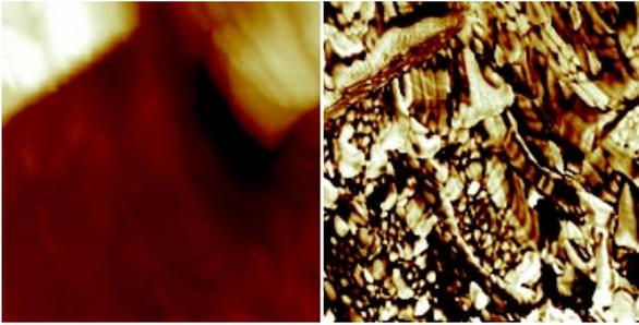
Figure 6: 2.5 $\mu\text{m}$  images of a quartz crucible used to grow crystalline silicon at high temperature. The multi-component structure in the phase image (right) is likely caused by Si contamination of the crucible that prevents its re-use. Sample provided by Dr. Robert Fisher, University of Washington.
