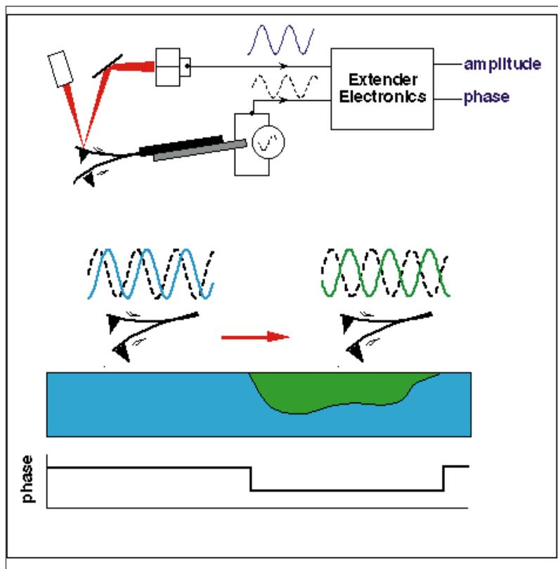
Figure 1: Phase imaging uses the Extender Electronics Module to measure the phase lag of the cantilever oscillation (solid wave) relative to the piezo drive (dashed wave). The amplitude signal is used simultaneously by the NanoScope III controller for TappingMode feedback. Spatial variations in sample properties cause shifts in the cantilever phase (bottom) which are mapped to produce the phase images shown here.
