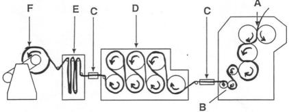
Figure 1.5 Schematic view of an inverted "L" calender plant for the production of plastic sheeting. Molten polymer is dropped into the calender system at A. Continuous sheet is formed by passing the melt between the rolls. One of the surfaces is given texture by an embossing roll, B. Thickness gauges, C, provide data for control of the process. The sheet is cooled, D, tensioned using wind-up accumulators, E, and accumulated on the wind-up roll, F (Holmes-Walker, 1975).
