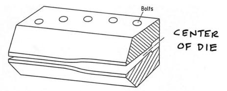
Clam shelling due to internal pressure in a flat slit die
