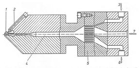
Fig. 6.2 Feed block (System Dow) for bringing melt streams together before the flat slit die. I Flex lip, 2 Pressure bolt, 3 Cover layer material, 4 Melt channel with a flow restrictor, 5 Adapter, 6 Base layer material, 7 Main layer material
