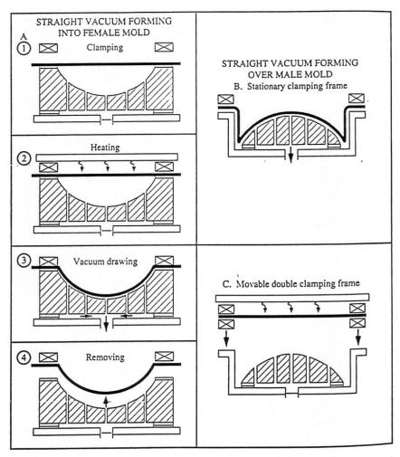
Fig. 10-8 Methods of straight vacuum forming [2].
