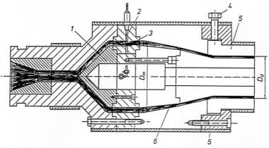
Mandrel support die (principle). 1 Mandrel tip, 2 Mandrel support, 3 Spider leg, 4 Centering screw, 5 Die ring, 6 Relaxation zone
