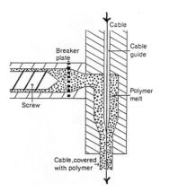
Combination of Poiseuille flow (pressure driven) and Couette (drag) flow due to the moving wire. More on Wire-Coating in the NEXT LECTURE
