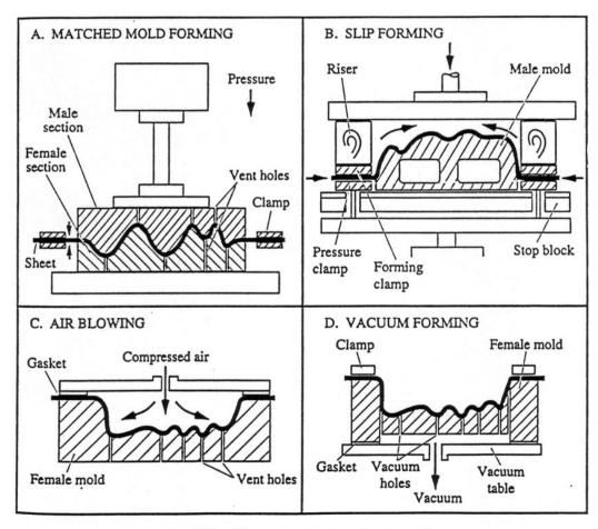
Fig. 10-2 Thermoforming classifications [2].
