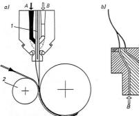
Dual slot coextrusion dies, a) Flat slit die, 1 Heat separation, 2 Pressure roll, b) Blown film die
