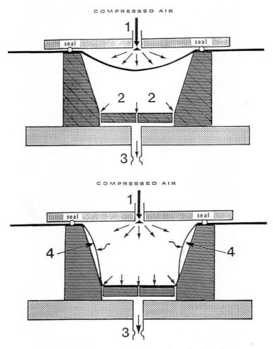
FIGURE 76 Overpressurized forming condition: (1) incoming pressure force; (2) undersized or small number of vent/vacuum holes; (3) restricted vent/vacuum channel; (4) trapped air pockets.
