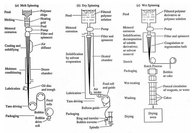
Fig. 11-1 Schematic diagrams of spinning processes [1].
