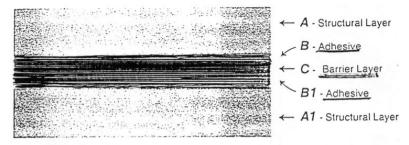
Figure 5-2 Typical structure of a five-layer coextrusion. Courtesy: Dow Chemical Company.
