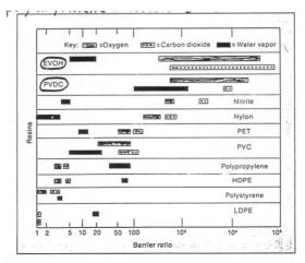
Figure 5-5 Comparison of barrier properties of various polymers used in packaging. <u>Barrier ratio-thickness ratio to reach equivalent barrier</u>. Courtesy: *Plastics Engineering* (May 1986).
