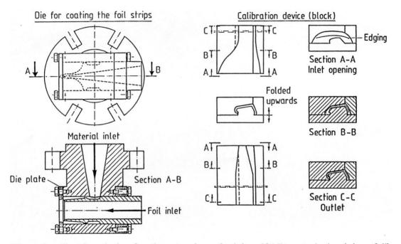
Die and calibration device for the extrusion of edging (CAB coated aluminium foil]
