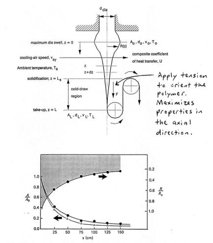
**Fig. 15.1** Melt strand area and radius profiles in the melt drawdown region:  $\bullet$ , nylon 6 at 265°C and takeup velocity of 300 m/min;  $\triangle$ , PP at 262°C and takeup velocity of 350 m/min. (Reprinted with permission from H. F. Mark, in *Rheology*, Vol. 4, F. R. Eirich, ed., Academic Press, New York, 1969.)
