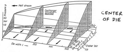
Typical pressure distribution in a flat slit die
