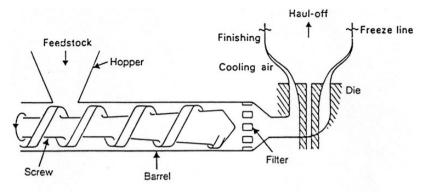
Fig. 7.1. Extruder and die in a film blowing unit (after Cogswell).
