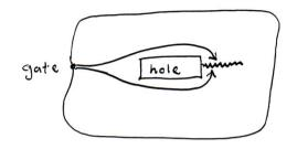
Figure 7: Cold flow fronts recombine to make a visible line that can be mechanically weak.
