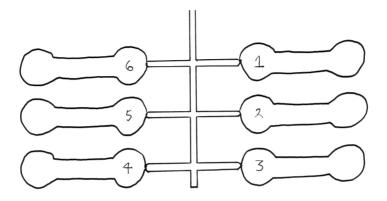
Figure 3: Need to **overpack** 1 and 6 to fill 3 and 4.
