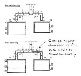
Figure 2: An artificially balanced runner system.
