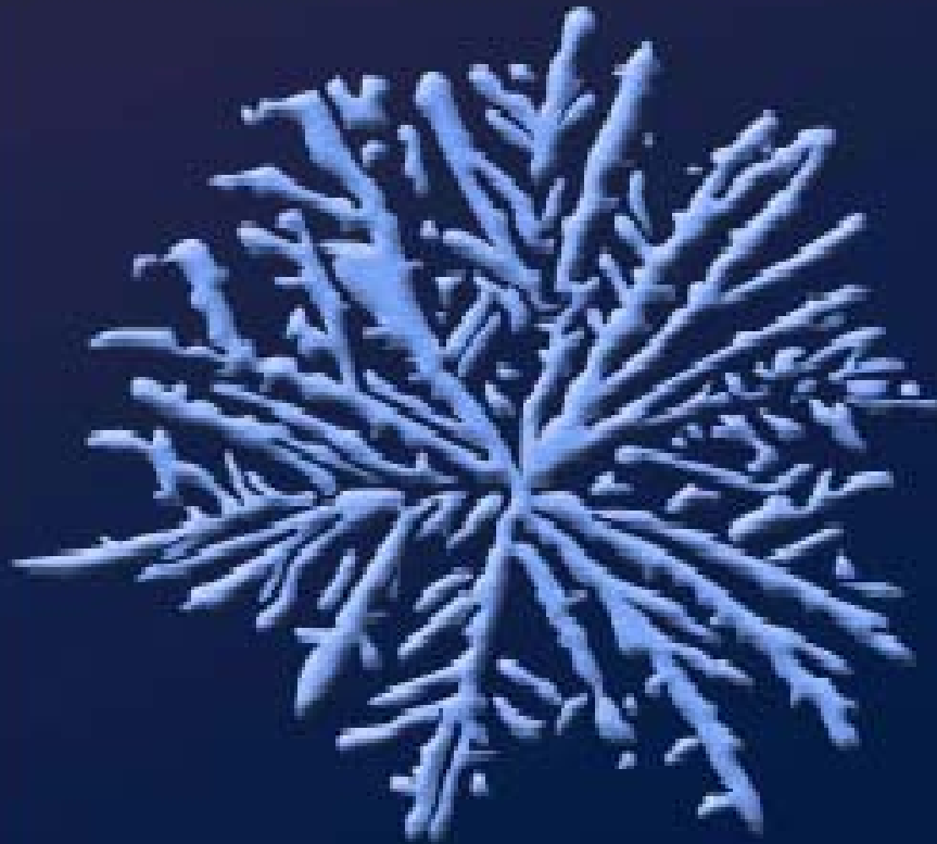
IPP Spherulite grown from a 10% IPP, 90% APP mixture
