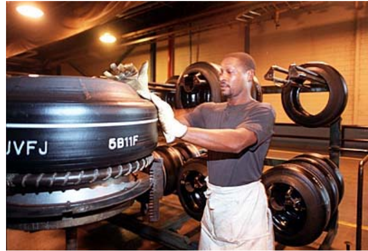
Firestone/Bridgestone truck tire prior to curing
